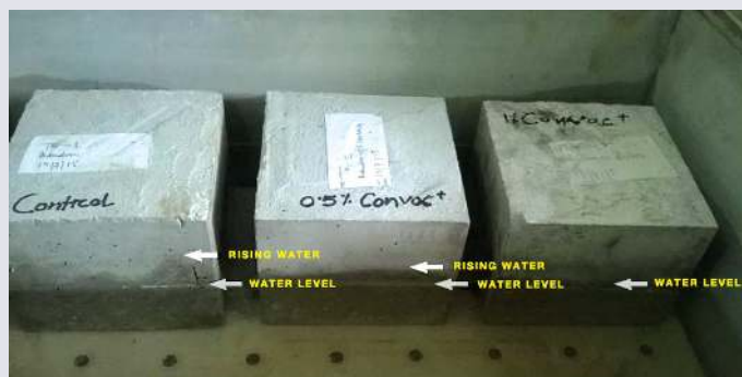
Rising Damp Test on Concrete Cube: Rising Damp is almost nil with the use of CONVAC PLUS (dosage of 1% BOWC)
